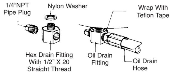
5. Locate drain hose on vertical bulkhead or firewall and secure with plastic hose hanger. Do not kink hose or locate so that it touches the engine. See that all fittings are tightened securely. Installation is now complete.
