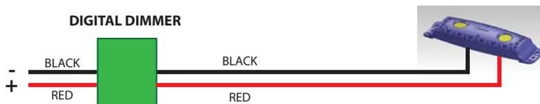
*Reversing the polarity (2 wire setup) - HI / LO capability*
