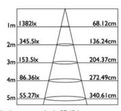
Height Emax Angle:37.62deg Diameter
