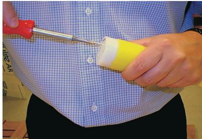
**5** Tighten down the recessed screws with moderate torque.
