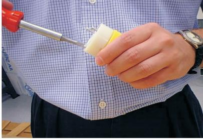
**1** Back out the three recessed screws and separate sections.
