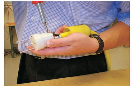
**3** Insert bare wires into their corresponding color-coded terminals. Make certain there is not wire insulation under any terminal clamp. Tighten the screw clamps to 14-20 inch-pounds torque.
