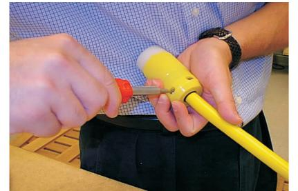
**6** Tighten cord clamp by tighten two assembly screws to 16-20 inch-pounds torque.
