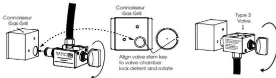
Insert valve as shown in diagram above. Valve may seem loose, this is OK. Valve does not have to be snug-fitting to be safe or function properly.
