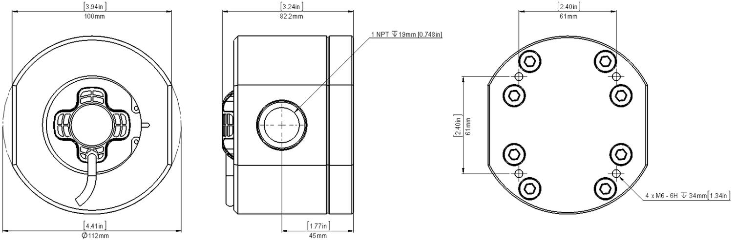
**Figure 3 - Fuel Flow Sensor Mechanical Drawing**
