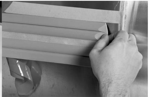
Once fully attached, use the burnishing tool to apply additional pressure to the entire PontoonGuard, ensuring the pressure sensitive adhesive is firmly attached.
