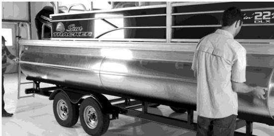
Measure the length of the pontoon tube. If the PontoonGuard is too long, trim the PontoonGuard with a utility knife on the rear squared edge for a precise fit.
