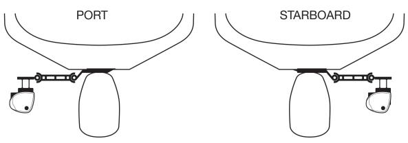
**NOTE:** IF AN ADAPTER BRACKET NEEDS TO BE MOUNTED TO BOTH THE PORT AND STARBOARD SIDE, THE SHIM BRACKETS WILL NOT BE USED AND WILL BE REPLACED WITH ANOTHER ADAPTER BRACKET FOR THAT SIDE. IF THE BOAT IS TO BE RIGGED THAT WAY, IT MAY BE NECESSARY TO REMOVE A FACTORY EQUIPPED E-LADDER FOR PROPER BRACKET INSTALLATION. DUE TO THE WIDE VARIETY OF E-LADDERS, MINN KOTA IS NOT RESPONSIBLE FOR THE RE-INSTALLATION OR RE-LOCATION OF ANY FACTORY EQUIPED E-LADDER.
