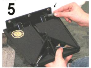
Attach the Plate: Align the plate & hinge holes, and use the 3/8" diameter 'snap & lock' pins to secure the plate to the hinge. Push the pins in until the head is flush. This may take some effort.
