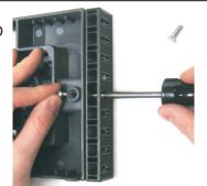
3. WITH SPRING WEDGED IN PLACE, ATTACH (N) SCREW THROUGH COUNTERSUNK HOLE. ONCE TIGHTENED, REMOVE (K) SCREW FROM SPRING.
