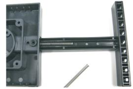
2. COMPRESS SPRING INTO TRAY USING A PHILIPS HEAD SCREW DRIVER. WHEN SPRING REACHES PAST COUNTERSUNK HOLE, WEDGE SPRING IN PLACE WITH (K) SCREW.
