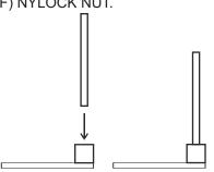
2. LOCATE THE ATTACHMENT POINT THAT WILL SECURE YOUR RAM® POD I™. START WITH THE BASE END AND BEND THE (A) FLEX ROD USING TIGHT BENDS, AND CONTINUE TO SHAPE THE ARM UNTIL IT REACHES ITS APPROXIMATE LOCATION
