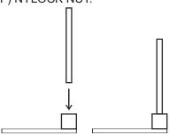
2. LOCATE THE ATTACHMENT POINT THAT WILL SECURE YOUR RAM® POD I™. START WITH THE BASE END AND BEND THE (A) FLEX ROD USING TIGHT BENDS, AND CONTINUE TO SHAPE THE ARM UNTIL IT REACHES ITS APPROXIMATE LOCATION
