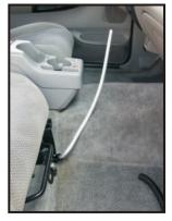
3. SLIDE (B) TUBE COVERING ONTO (A) FLEX ROD. INSTALL (C) PIPE CLEVIS ON TOP OF FLEX ROD AND SECURE USING (G) MACHINE SCREW AND (H) NUT.
