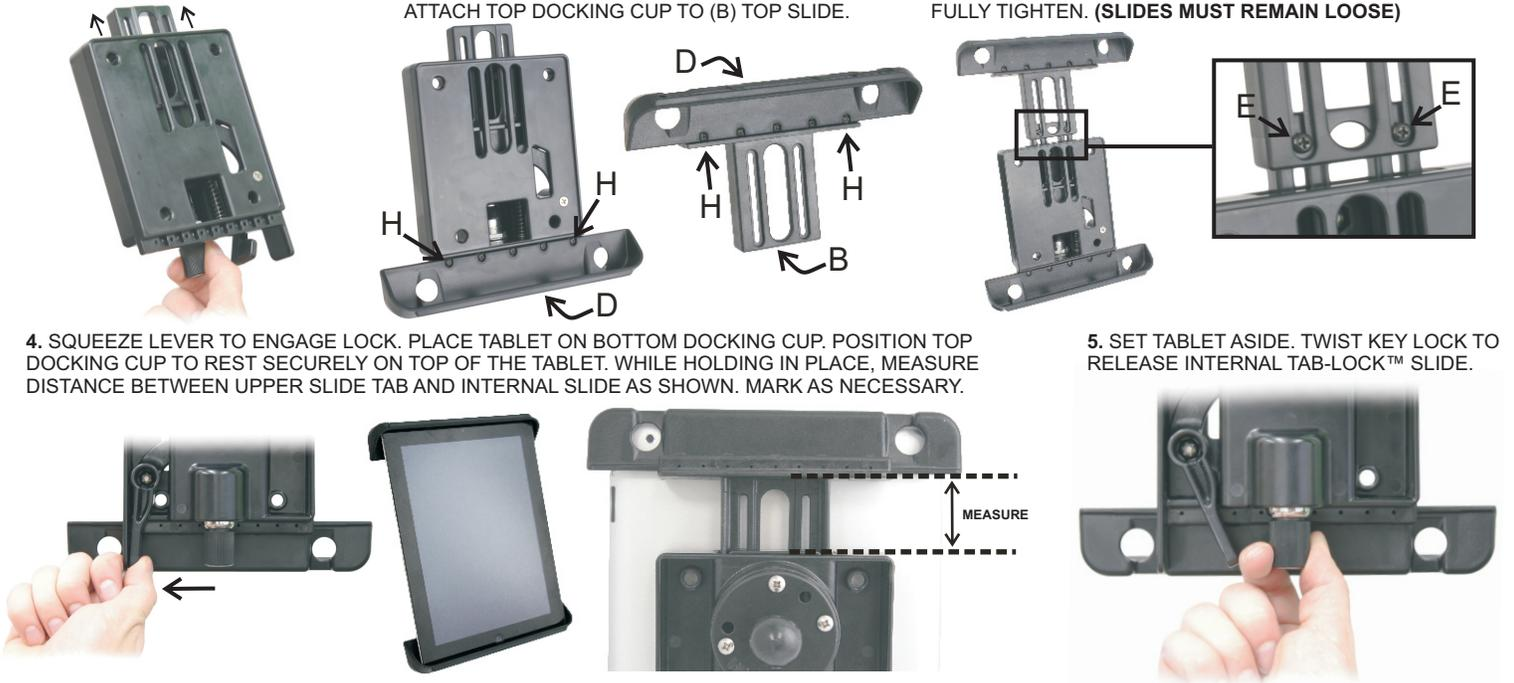
4. SQUEEZE LEVER TO ENGAGE LOCK. PLACE TABLET ON BOTTOM DOCKING CUP. POSITION TOP DOCKING CUP TO REST SECURELY ON TOP OF THE TABLET. WHILE HOLDING IN PLACE, MEASURE DISTANCE BETWEEN UPPER SLIDE TAB AND INTERNAL SLIDE AS SHOWN. MARK AS NECESSARY.
