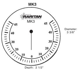
Select an area where the Ruddermaster can be easily viewed by the navigator, but also where the Ruddermaster will not be affected by washdown spray or by direct elements. Ruddermasters are not water resistant except for the MK2 and MK3 which are spray proof (IP64).
