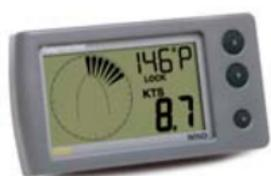
ST40 Wind instrument features wind speed and direction in both apparent and true. Wind angle can be locked manually or automatically. Display features: Deviation and course-to-steer to achieve locked wind angle. System supplied with rotavecta type wind transducer.
