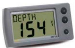
The ST40 Depth instrument is available as a system with a transducer or as a repeater display. Display features: 200Khz frequency, digital depth display of minimum depth, shallow and deep anchor alarms. Depth can be displayed in feet (ft), meters (m) or fathoms (fa).
