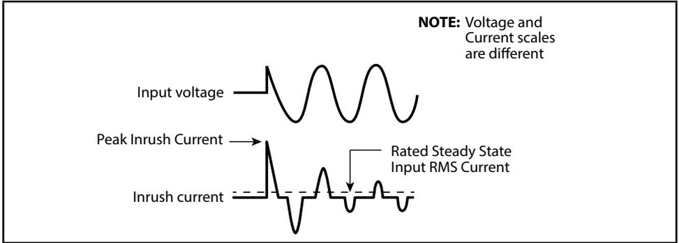
Fig 1.2 Inrush current in an SMPS
