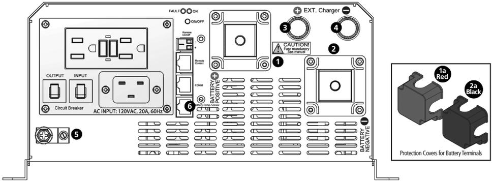
Fig 3.8 DC Side Connections
