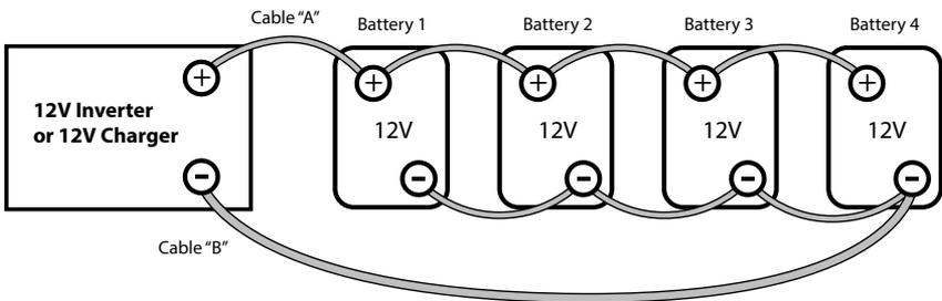
Fig 3.6 Parallel Connection
