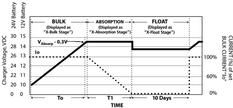
Fig 5.1 Charging Curves for 3 Stage Charging Profile
