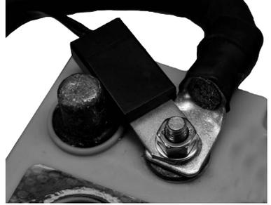
Fig 2.5(b) Temperature Sensor Installation
