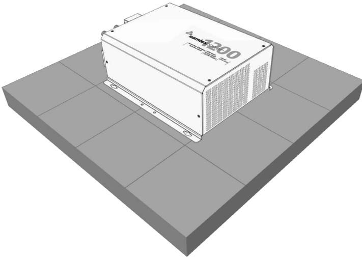
**Fig 3.2 Mounting Arrangement No.1: Horizontally On Horizontal Surface**
