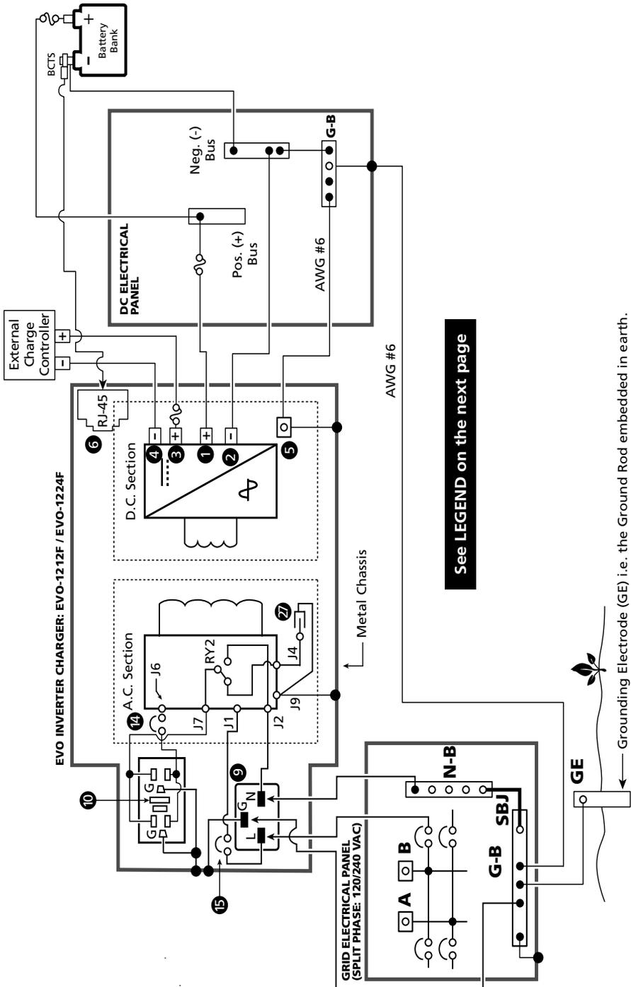
Fig 3-12 Installation Diagram for Typical Shore Based Installation for EVO-1212F and EVO-1224F
