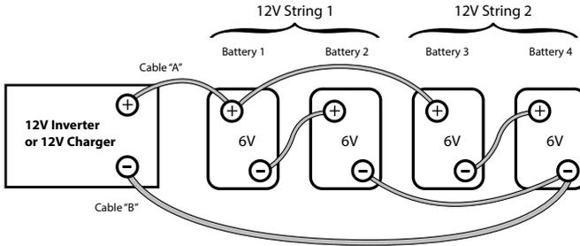
**Fig. 3.7 Series-Parallel Connection**
