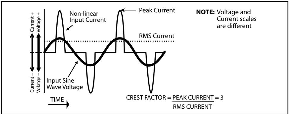
Fig 1.3 High Crest Factor of current drawn by SMPS
