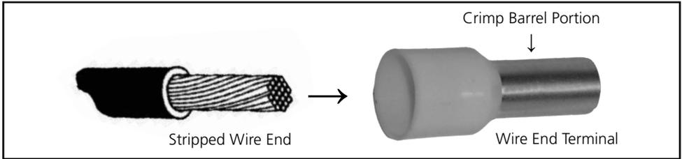
Fig 3.11 Stripped Wire End Terminal on AC Wiring
