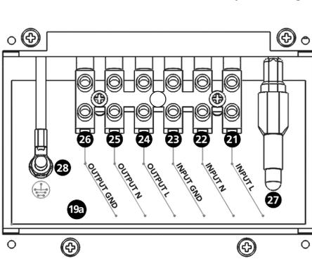
**Fig 3.9.2(a) Pocket for AC Input and Output Connections for EVO-1212F-HW and EVO1224F-HW**
