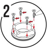
Drill pilot holes and secure the base. Apply marine adhesive sealant to the threads of the screws.
