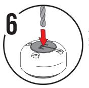
When drilling, the drill should be run repeatedly through rubber.
