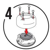
Line up the Cable Gland cover with the four holes in the plastic base and screw the bolts in with a 2.5mm wrench, compressing the rubber grommet.
