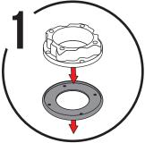
Place the plastic base onto the rubber base gasket. Be sure to line up the four screw holes.
