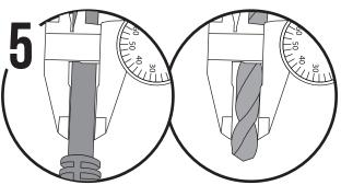
Measure your cable diameter and select the appropriate drill bit. For a 0.25" cable use a 9/32" or 7mm drill bit. For a 0.40" cable use a 7/16" or 11mm drill bit.
