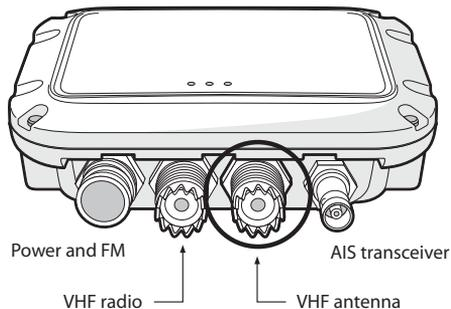
Figure 6 Position of the VHF antenna connector
