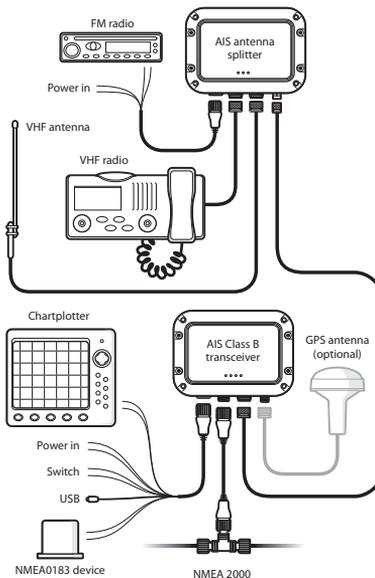
Figure 3 Typical installation configuration
