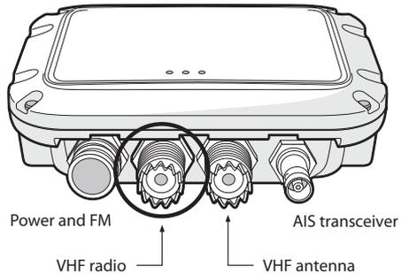
Figure 7 Position of the VHF radio connector
