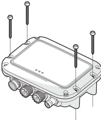
Figure 5 AIS antenna splitter mounting
