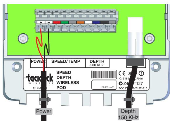
**GB To install Raymarine (Airmar) 200 KHz transducers:** Connect the transducer cables, following the colour coding on the Pod. Sheath the screens to avoid short circuits. **Note:** For best performance, cut the 200 KHz signal cables as short as possible.
