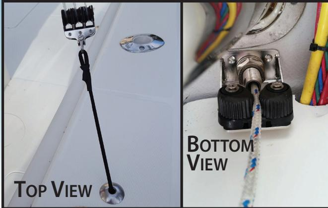
The Taco Marine Outrigger Line Tensioner is designed for larger boats that are fishing with double or triple lines on each outrigger. Outrigger Line Tensioners have been around for years in many shapes and sizes and are ideal for large center consoles or sport fishing boats. The purpose and function is to keep the proper tension on the outrigger lines and maintain them fully extended and tight.
