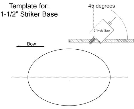
Warning: Do not drill bolts untill the lower base is flush to the deck surface
