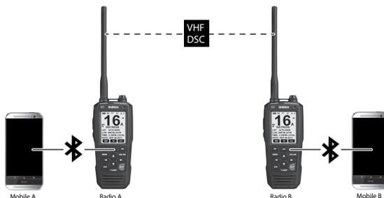
Enter text on Mobile A. Mobile A transmits to Radio A through Bluetooth. Radio A transmits to Radio B through VHF DSC. Radio B transmits to Mobile B through Bluetooth.
