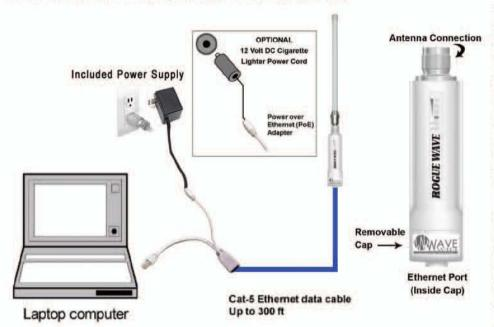
Secure the antenna supplied with the kit to the Rogue's 'N' connector. Unscrew the protective cap from the other end of the Rogue and pass one end of the supplied Ethernet cable through the cap. Plug the Ethernet cable into the Rogue and securely replace the cap inserting the rubber grommet around the cable and the cap.
