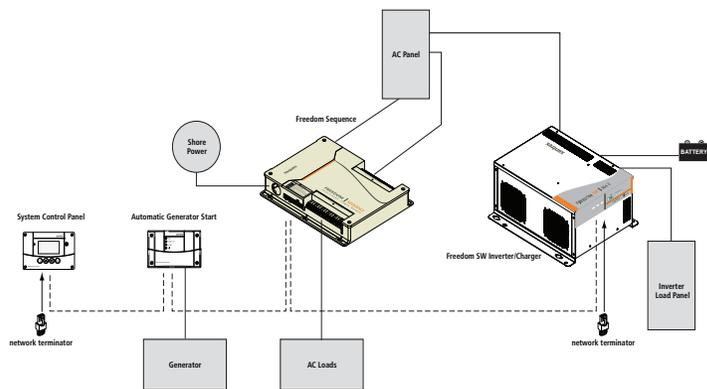
Figure 1 Typical Xanbus System Diagram
