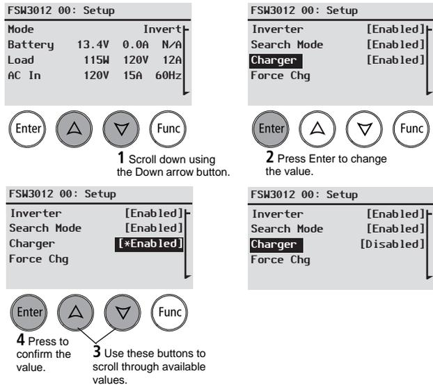
**Figure 20** Selecting and Changing a Configurable Setting
