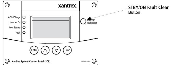
**Figure 14** Xanbus SCP STBY/ON Fault Clear Button
