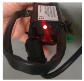
Check Incoming Data to make sure that Yamaha's (CPAC) three proprietary PGNs (065280, 127237 and 127245) are being received from the gateway. These three PGN's should be highlighted in reverse video. If they are light grey there is a problem with the network. Check to make sure you have a red light on the gateway and ensure you have a proper CAN bus network, such as 2 terminating resistors.
