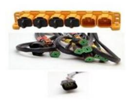
(3) Disconnect the multi-link cable connector and install the Y-split cable for multi-link cable installation or if there is a hub simply plug the Helm Master gateway into the open port on the hub and disregard the Y-Split Cable.
