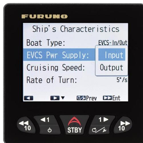
This completes the NavPilot 300 initial settings for use with a Seastar Optimus steering system. Other basic NavPilot 300 settings still need to be set, such as the **Heading source**, **Position source**, etc.
