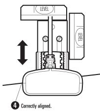
**Downward Slant:** The transducer has a natural downward slant of 4 to 5 degrees from leading edge to trailing edge. Looking at the back of the transducer, the seam should be slightly below the bottom of the hull.
