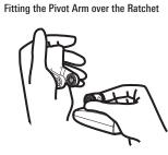
NOTE: The ratchets are keyed. Make sure that the square teeth on each ratchet face the square teeth on the transducer knuckle, and the triangular teeth face outward.
