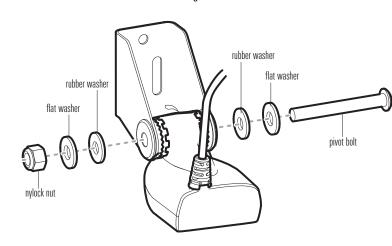
5. Align the mounting bracket transducer assembly with the drilled holes in the transom. With a 5/16" (8 mm) socket driver, mount the assembly to the transom using the two #10 - 1" (25.4 mm) long screws provided. Hand-tighten only!
