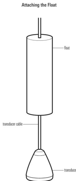
2. Position the float so that the transducer will be submerged in the water, just below the ice.
