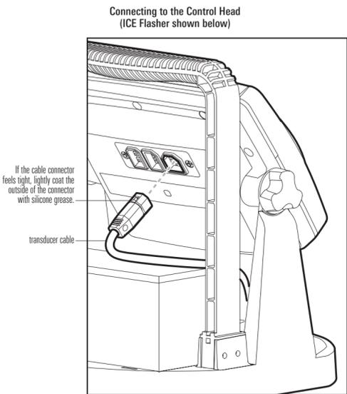
**NOTE:** If you have an ICE 55 Flasher, remove the control head and base from the portable bag to connect the transducer cable, then reinstall it in the portable bag.
