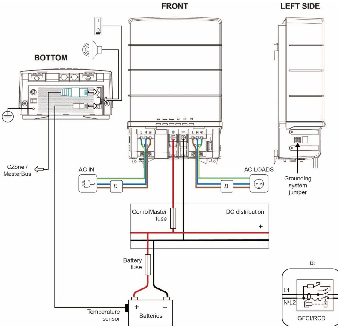
Figure 3: Installation drawing CombiMaster Inverter/Charger
