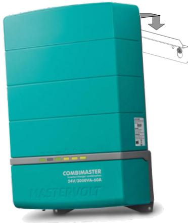
**Step 4.** Fix the CombiMaster Inverter/Charger to the surface by fastening two screws at the lower side of the case as well.
