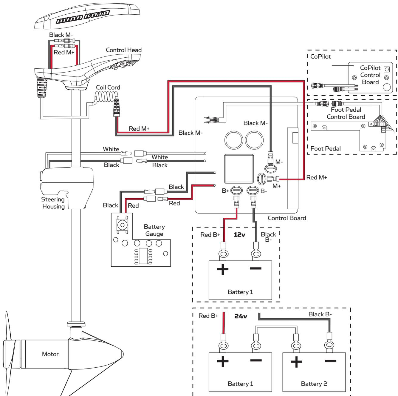
**NOTE:** This is a multi-voltage diagram. Double-check your motor's voltage for proper connections. Over-Current Protection Devices are not shown in this illustration.
