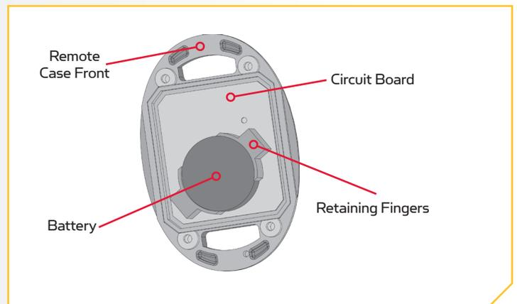
**NOTE:** The replacement battery must be a model CR2032 coin cell type. It is strongly recommended that a name brand battery is used.
