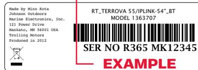
**NOTE:** The serial number on your Riptide Terrova is located inside the mount below the motor rests.
