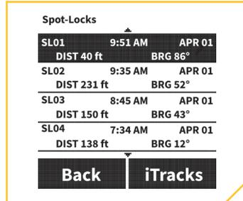
A list of Spot-Locks that are in navigable range. The date and time listed are generated when the Spot-Lock is saved.
