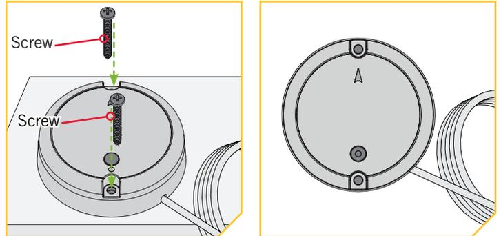
**NOTICE:** If replacement screws must be used, ensure that they are high grade non-magnetic stainless steel.
