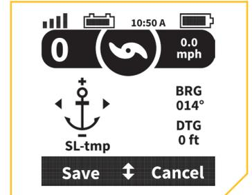
A temporary Spot-Lock created when the Spot-Lock button is pressed and Spot-Lock Jog is available.
