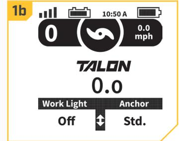
**NOTICE:** When the i-Pilot System is paired with two Talons, toggling the Anchor Mode on the i-Pilot Remote for one Talon will toggle the Anchor Mode for both Talons.
