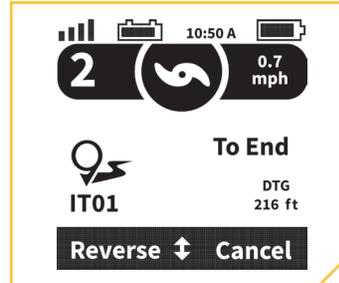
Navigating an iTrack when the boat is on course to go to the end of the iTrack.
