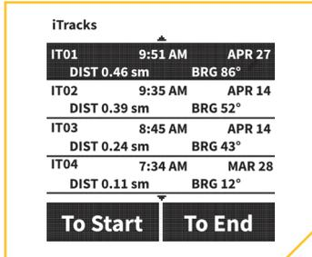
A list of iTracks that are in navigable range. The date and time listed are generated when the track is recorded.
