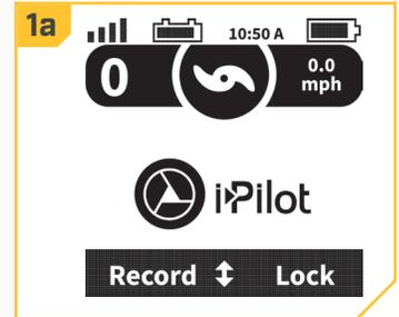
**NOTICE:** When the i-Pilot System is paired with two Talons, toggling the Work Light Intensity on one Talon will toggle the Work Light Intensity on both.
