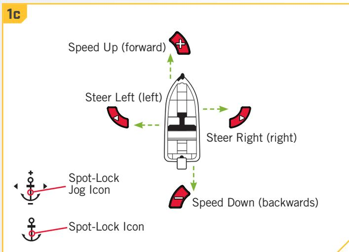
**NOTICE:** A Heading Sensor is required for Spot-Lock Jog. If your motor is not paired with a Heading Sensor, the Spot Lock icon will appear without the directional indicators and the option to jog will not be available.
