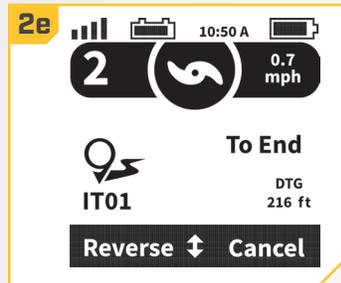
**NOTICE:** If Auto Prop On is turned "off" the prop must be enabled before the boat will begin navigating an iTrack.
