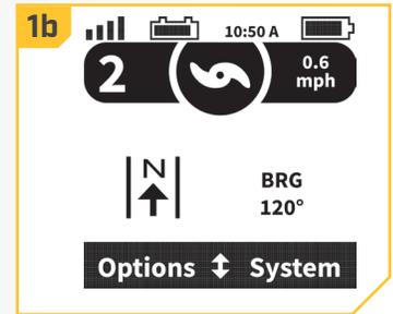
**NOTICE:** After steering to a new direction, there is a short delay before the direction is locked in to allow the compass to stabilize. When broad speed changes are made, the motor heading may change slightly. This is normal.
