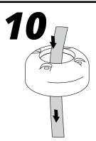
Slide the Cable Gland cover over the electronic cable.
