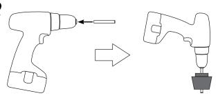
Insert drill tube into drill motor, and leave enough length to get through the tapered plug.
