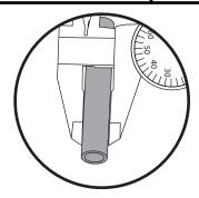
Measure your cable diameter and select the appropriate drill tube provided.
