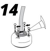
Apply marine adhesive sealant to the four allen head screws and tighten.
