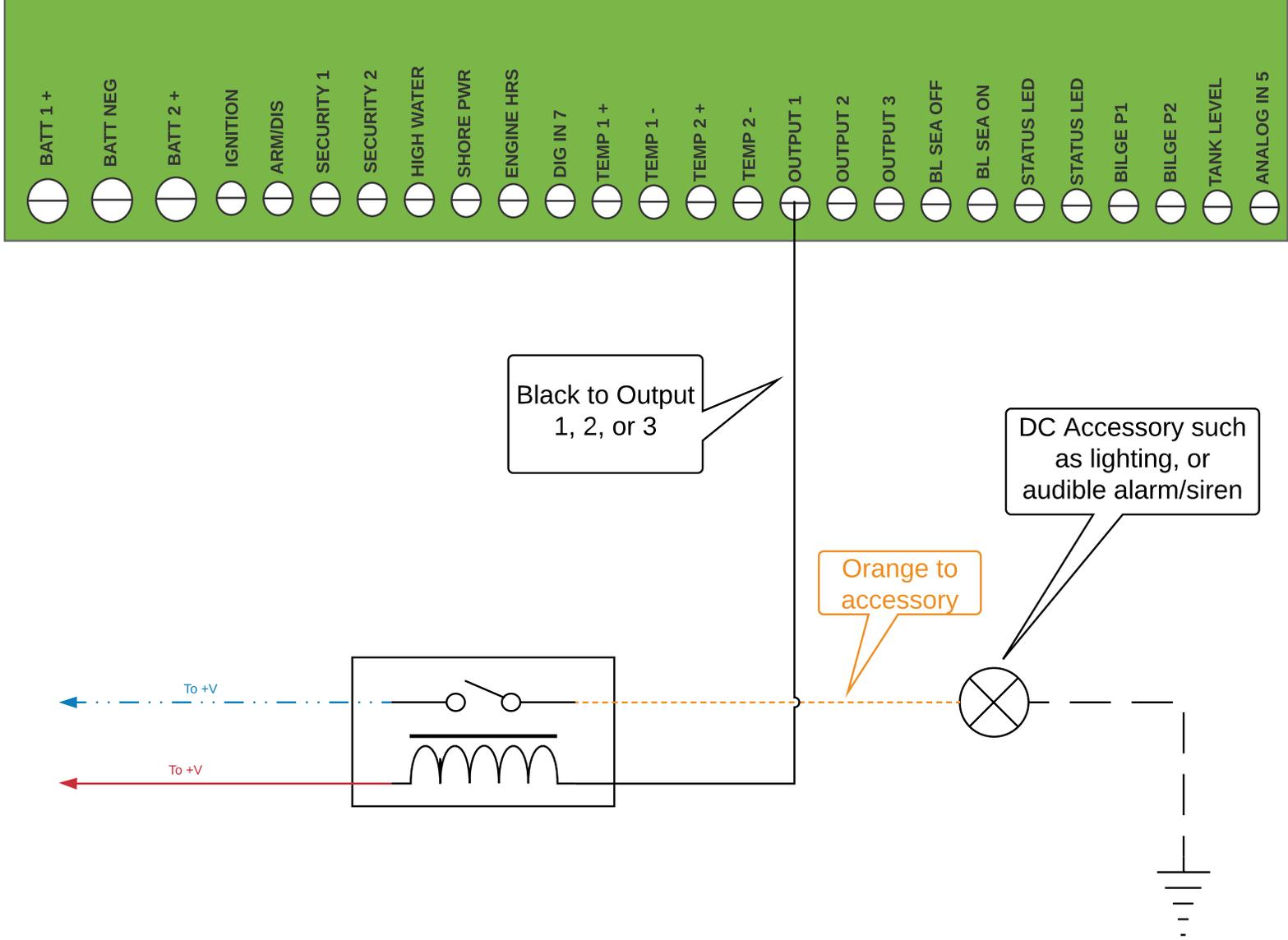
To use the MTC for remote switching using Outputs 1,2, and/or 3 a relay is needed. The Siren Marine DC Relay (PAM-4) meets this need for most DC accessories. *Outputs 1,2, and 3 are rated for 1 amp.*
