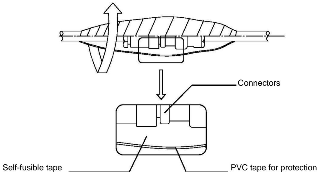
**Figure 7.5 Processing on the coax cable jointing section**
