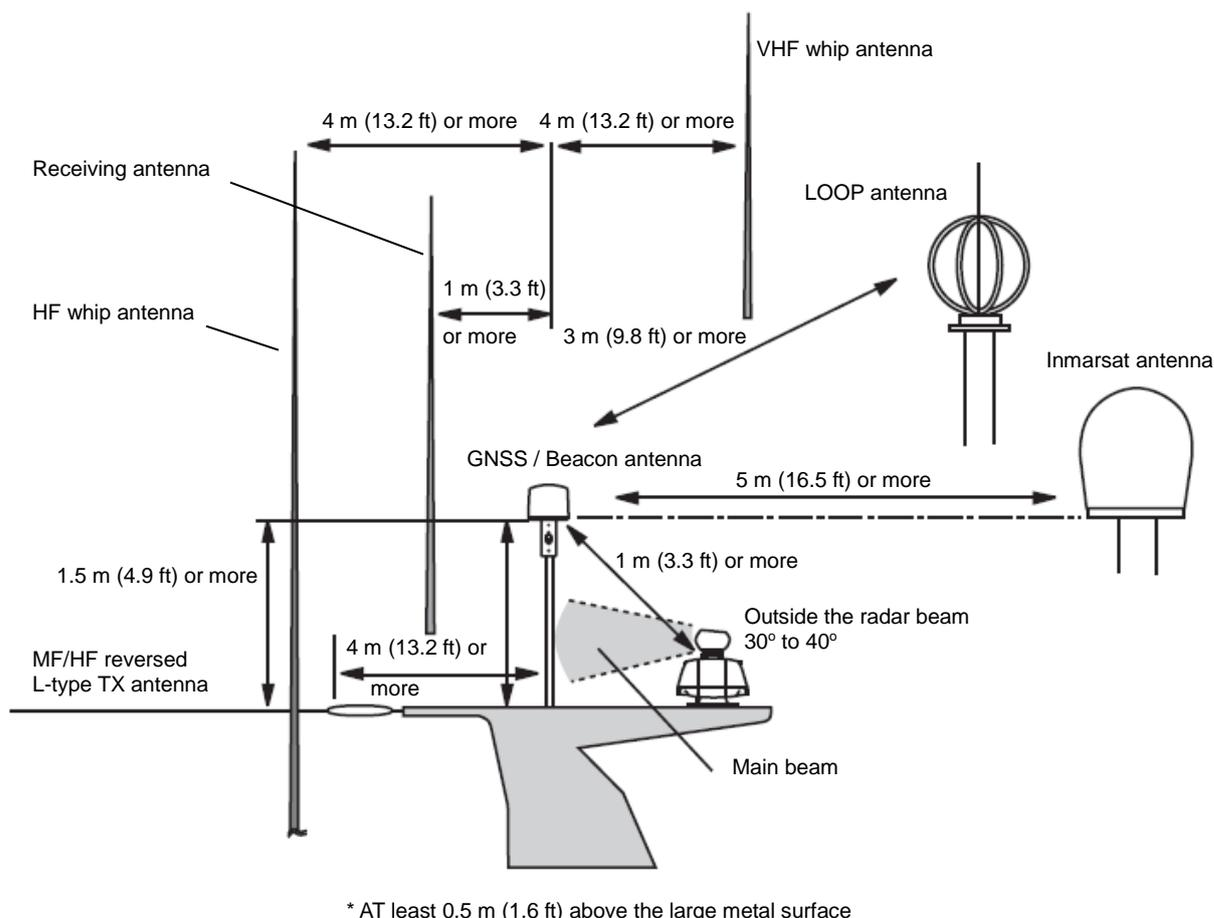
**Figure 7.4 Recommended GPS / Beacon Antenna installation**
