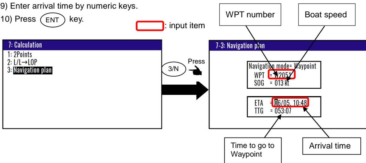
**Calculating arrival time and total navigation time from route plan and boat speed**
