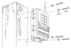
the holes at the bottom of the shelter into the post. Using an adjustable wrench or 7/16" wrench, tighten the lag screws.
