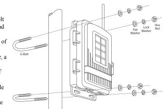
4. Place the second U-bolt around the pole and through the two holes at the bottom of the shelter. Put a flat washer, a lock washer, and a hex nut on each bolt end, and tighten the hex nuts.
