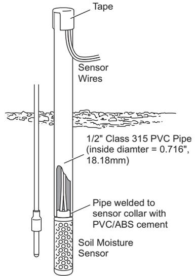
4. Carefully backfill the access hole with soil to eliminate any air pockets which could allow water to channel down to the sensor.
