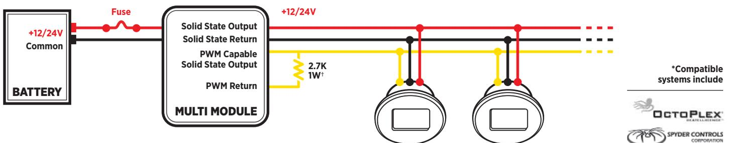
\* By driving the Yellow wire Low (i.e. DC Common), the Fixture turns off. Many Multiplex type systems were originally designed for halogen lamps and do not Drive Low, in which case in this example a 2.7K, 1 Watt Pull Down Resistor pulls down the Yellow Dimming Line to DC Common when the PWM is not driven High (thus shutting off the Fixtures).
