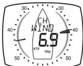
The true wind angle with respect to the vessel and the true wind speed calculated by the display taking into account the vessels speed through the water. Apparent wind speed, angle and boat speed must be available for this calculation. The wind angle is displayed on a 26 to 60 degree scale.
