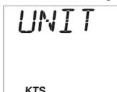
Sets the units in which all Wind Speed related information is displayed. **KTS (Knots)** or M/S (meters per second).
