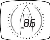
The windspeed over the ground is displayed in the Beaufort scale and in knots.
