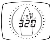
The compass heading that the vessel will follow should it tack through the wind, calculated by the display. Apparent wind angle and magnetic heading must be available for this calculation to be made.
