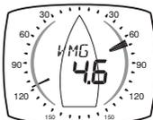
True wind angle (see above) is displayed on a 360 degree scale.
