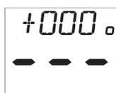
Aligns the displayed apparent wind angle with the actual wind direction with respect to the boat. See page 18 for calibration.
