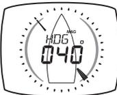
The current compass heading of the vessel as measured by the Compass Transducer.
