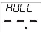
Shows the software version (before the decimal point), signal strength (after the decimal point) and battery condition (level and charge rate) of the Hull Transmitter to assist in trouble shooting and fault finding.
