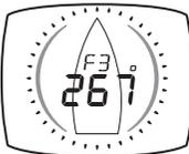
The true wind speed and direction over the ground are displayed using the Beaufort scale, calculated by the display taking into account the vessels speed through the water and compass heading.
