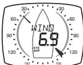
The apparent wind angle and speed with respect to the vessel as measured by the Wind Transmitter.
