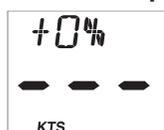
Adds a percentage factor which corrects the information from the Wind Transmitter and ensures the Apparent Wind Speed is displayed correctly. See page 18 for calibration.
