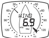
The true wind angle with respect to the vessel and the true wind speed calculated by the display taking into account the vessels speed through the water. Apparent wind speed, angle and boat speed must be available for this calculation. The wind angle is shown on a 360 degree scale.
