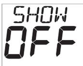
Allows the display of information when NOT installed as part of a Micronet system for demonstration purposes only.
