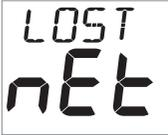
Indicates that the display has lost communication with the master. Either there is a problem with the master\* or the display has been moved out of effective range. The display will power down shortly after sounding the alarm in order to conserve power.
