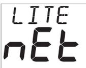
Tells the display to control the system Backlighting or just its own Backlighting. **nEt (network )** / LOC (local).
