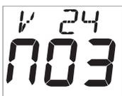
Shows the display's software version, battery level and charge rate to assist in troubleshooting and fault finding.
