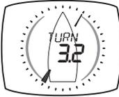
The pointer shows the direction of the target waypoint relative to the bow of the boat.
