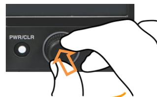
Push the rotary knob or tap the return icon to fix the setting.
