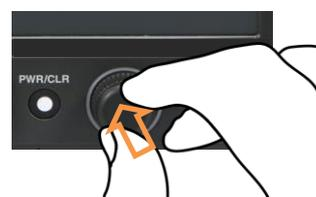
Push the rotary knob or tap the return icon to fix the setting.
