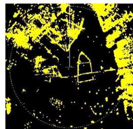
It is important to be note that if you adjust the gain level to maximum, the noise might be also displayed on the screen at the same time.
