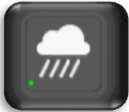
It is necessary to adjust the rain/snow clutter suppression level in order to use the radar exactly. Failure to do so, it is impossible to obtain an accurate radar echo.
