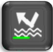
It is necessary to adjust the sea clutter suppression level in order to use the radar exactly. Failure to do so, it is possible to obtain an accurate radar echo.
