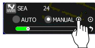
You should be adjust the sea level while monitoring the radar echo in TX mode.
