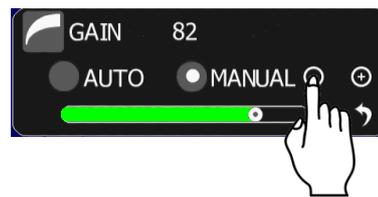
You should be adjust the gain level while monitoring the radar echo in TX mode.
