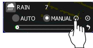
You should be adjust the rain/snow clutter suppression level while monitoring the radar echo in TX mode.
