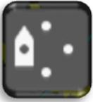
It is possible to shift the center of own ship in order to observe a particular target in a wider range. Be to tap once on the icon, center of own ship will be shifted as the following figures.
