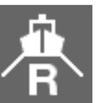
**Mode River:** Mode River is suitable for using river. This mode reduce sea clutter returns.
