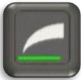
The gain level is displayed in the bottom portion of the icon. It is possible to judge the gain level by the length of a green bar roughly.
