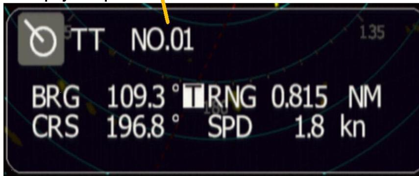
BRG: Target Bearing measured from own ship (True mode or Relative mode).
