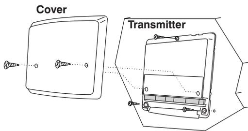
**GB** Mount at least 50cm above the waterline. Avoid direct contact with water. Mount in a well ventilated area. DO NOT mount in a sealed compartment. Mount the unit vertically, with the cables exiting at the bottom **Note:** the template must be inverted for Transmitters. Drill three 2.5mm holes marked "B" on the Template. Attach the Transmitter using the selftapping screws provided. **Warning:** do not over tighten the screws, this may cause the moulding to crack.
