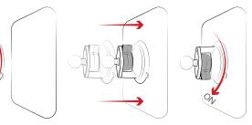
RAM<sup>®</sup> Twist-Lock<sup>™</sup> Suction Cups are only compatible with smooth, non-porous surfaces (no rough or textured surfaces). Clean surface thoroughly before applying suction. When left unattended in extreme temperatures. it is recommended to remove and stow suction cups. Suction cups are considered a general wear item and are not covered under any warranty.
