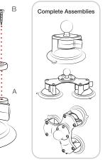
Clean surface thoroughly. Align the suction cup to surface. While holding the lever to the OFF position, push the plastic base onto the surface flush with the silicon base and switch the lever to the lock position. Suction cup base must be locked flush with the silicon for a successful hold.
