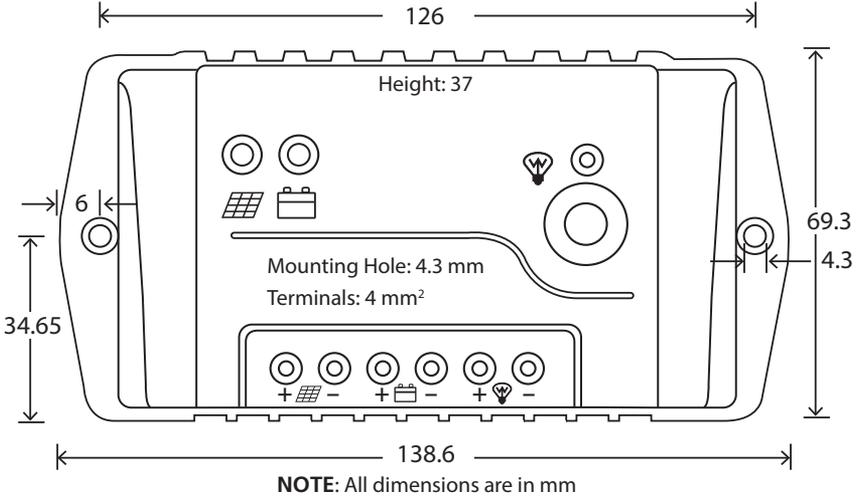
Fig 3.1: Dimensional Drawing of Charge Controller MSK-10A
