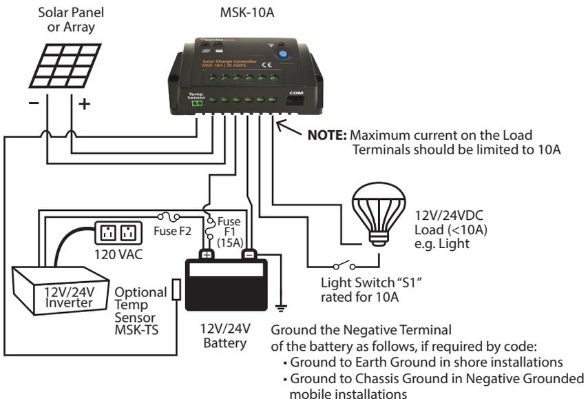
Fig 3.2: Wiring Diagram
