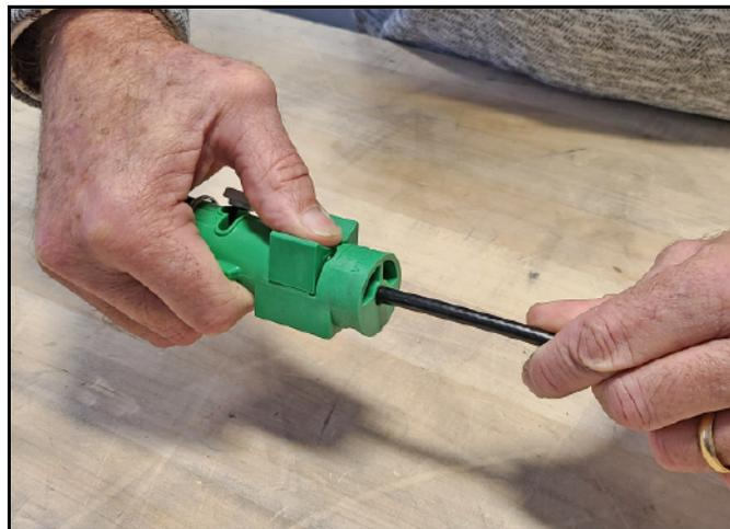
**Note:** Carefully remove any residual plastic from the center conductor, if necessary.
