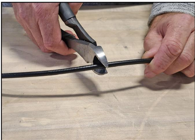
2. Since cutting the cable can deform the end, gently round the end of the cable. Also make sure the center conductor is centered within the cable.
