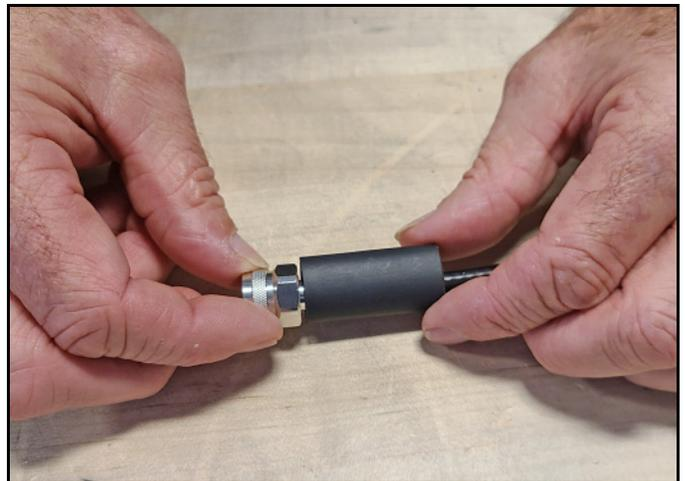
When you are done, the heat shrink should extend from the rear of the connector to the cable jacket. This forms a weather-tight seal.
