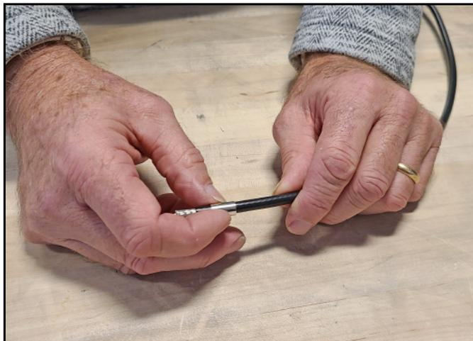
4. Insert the end of the cable into the #1 end of the CST-240 stripping tool. Depress the cutting blade using your thumb, then rotate the tool clockwise around the cable until the tool turns easily. The end of the cable should now be stripped to expose the center conductor.
