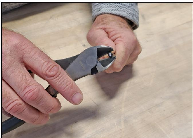
3. Place the metal ferrule onto the cable.
