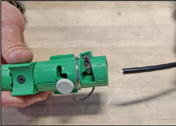
Figure 51: Cable Stripped, Exposing Dielectric
