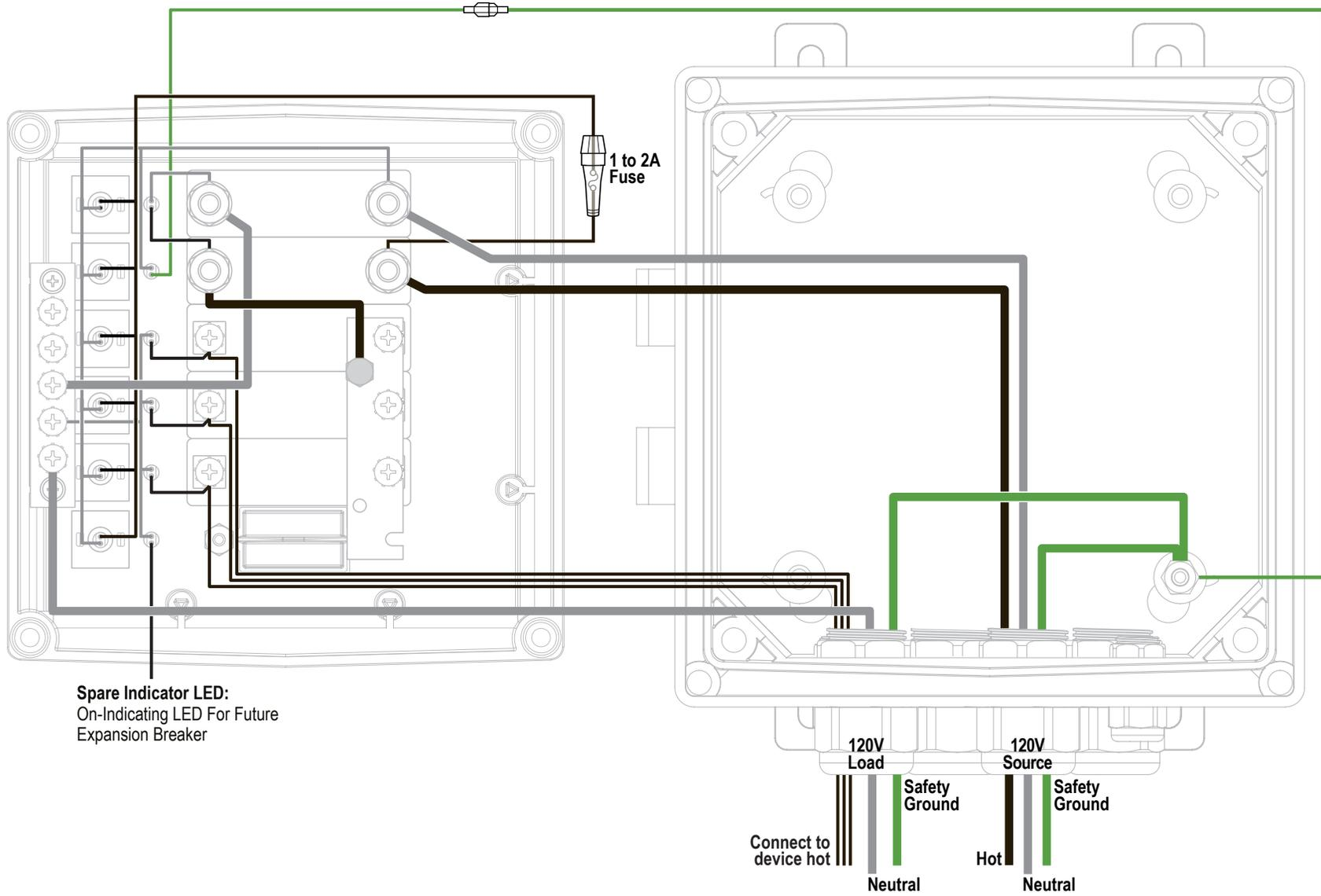
**SMS Enclosure Panel Assembly Wiring View**
