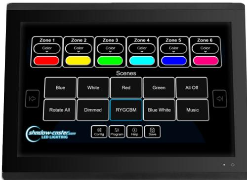
Connect to your compatible MFD and utilize Shadow-Caster®'s custom lighting interface to create lighting scenes, customize and name zones, and assign devices to zones. Compatible with Garmin, Simrad, Lowrance, B&G, Raymarine, and Furuno. **SCM-Light Commander Plus**
