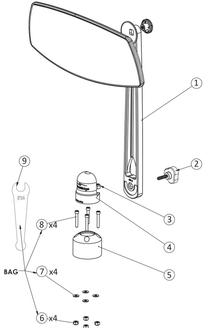
**TIP:** After tightening the knob in step 10, you can rotate the mirror arm clockwise even further (in the same direction as the knob) to ensure a more secure fit.
