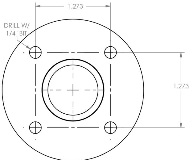
6. Use a 1/4" drill bit to drill the four mounting holes through the masking tape.
