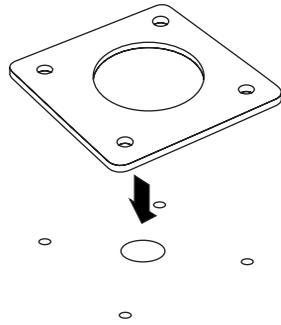
**12** Route the cabling through the center hole. Place the mount assembly on top of the foam gasket.
