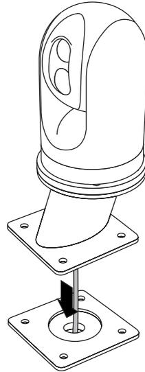
**13** Apply marine adhesive sealant onto the four nylon shoulder washers. Then insert the washers into the four bolt holes on the base of the Seaview mount.
