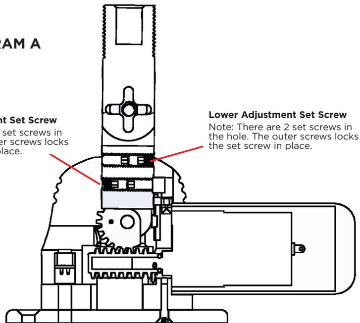
Adjustments to the arm position need to be done slowly 1/4 turn at a time. It is best practice to use an amp meter to determine when the sensor switch disables motor power. Failure to do this could result in motor failure.
