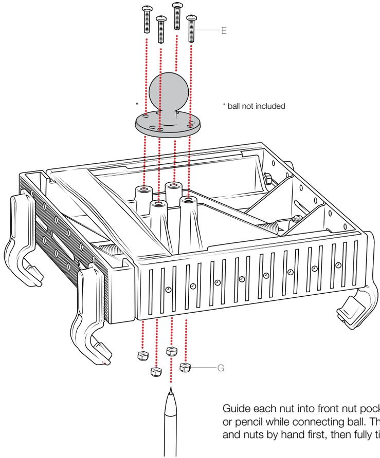
Guide each nut into front nut pockets with a pen or pencil while connecting ball. Thread all screws and nuts by hand first, then fully tighten.
